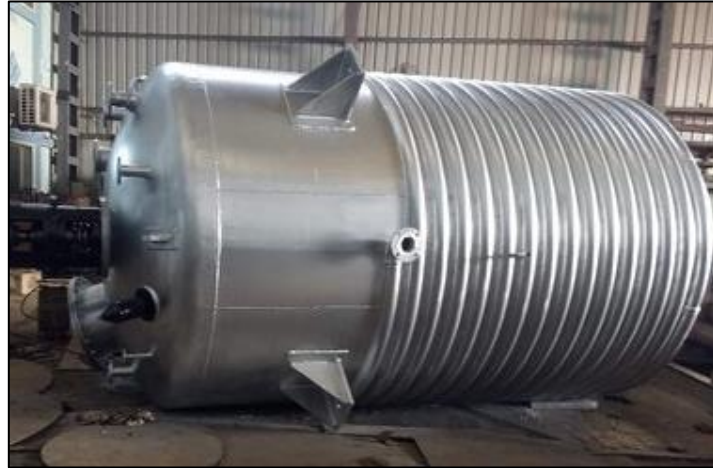
Fig.: polymerization reactor
