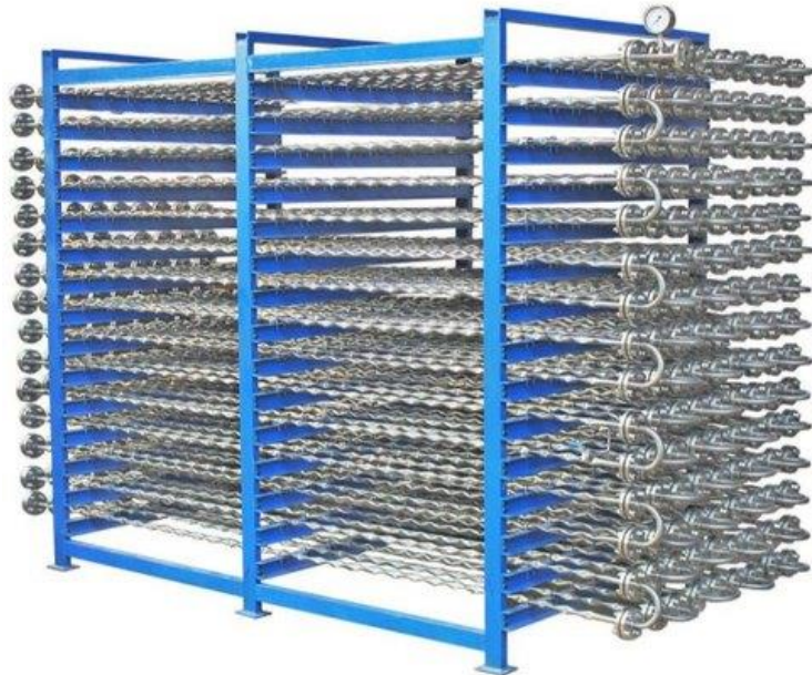
Fig.: plug flow reactor
